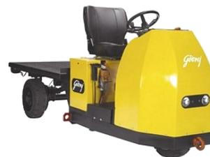
want to load / unload the platform manually. A 36V, 315 Ah battery means you can comfortably use the Platform Truck to carry loads up
