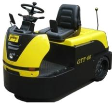
and economical to load them into trolleys and tow the trolleys to the desired location. For instance, carrying batches of machined parts from one processing section to another in an automobile or auto component manufacturing facility. Or carrying textile materials between sheds in a textile plant. Or handling baggage at airports. Or shifting goods within a warehouse serving
